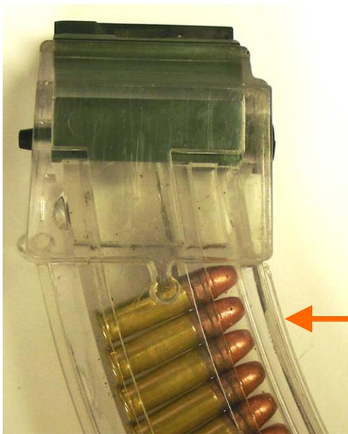
Check that ammunition doesn't bind in magazine
