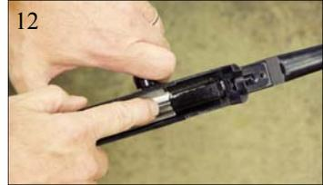
the kit handle moves forward it will interface with corresponding slot in the bolt and the bolt will drop down to its normal position. When this happens allow the entire bolt to move forward with it's own spring tension until it stops. NOTE: do not let the bolt slam forward without a barrel on the rifle, as it will mark the ejector port of the receiver.
