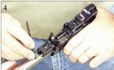
5. Position the safety halfway between on and off, then slip the stock onto the barreled 10/22 Action.
