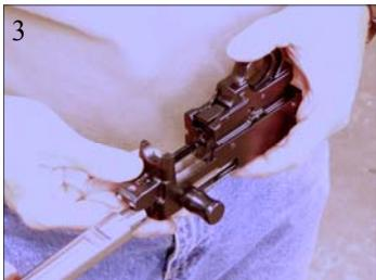
4. While holding the bolt slightly rearward (so that it won't be pressing against the barrel), tighten the V-Block retainer screws as shown below. Your new barrel is now installed!
