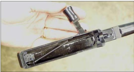
Installation of 17 HM2 Heavy Bolt Handle Assembly
