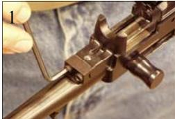
1. To remove the original barrel, locate the V-Block barrel retainer at the bottom of the barrel where it meets the receiver. Unscrew the two Allen screws.
