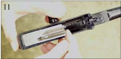
11. Once the bolt handle is all of the way back drop the rear of the bolt into the rear most part of the receiver and apply slight pressure down on the front of the bolt.
