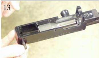
13. Install the largest of the three pins through the receiver.
