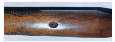
Drill the tuning access hole through the forend screw recess. Reattach your forend normally. Tune the Accurizer through the hole with an Allen® type hex wrench.
