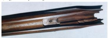
Use milling machine or Dremel with drum sander to inlet clearance for the Hicks #1 Accurizer in your forend.
